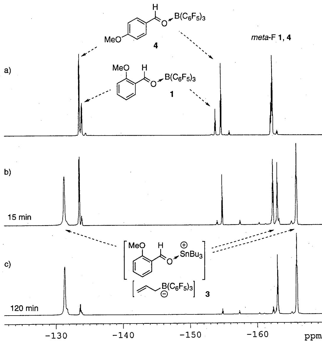
**Figure S2.** 282 MHz  $^{19}\text{F}$  NMR spectra ( $-60^\circ\text{C}$ ) of a) 1:1 *o/p*-anisaldehyde and 20%  $\text{B}(\text{C}_6\text{F}_5)_3$  (ratio of **4** to **1** = 2.4:1). b) Sample in a) 15 minutes after one equivalent of allyltributylstannane was added. Adduct **4** remains, while adduct **1** has been converted to ion pair **3**. c) Same sample 120 minutes after addition of allyltributylstannane. Conversion of the borane in the sample to ion pair **3** is complete.
